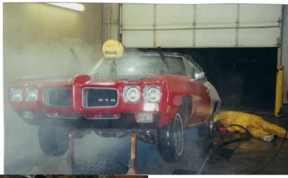
to pull the body off the frame. The body mounts looked pretty bad anyway, so I decided to go ahead and replace them all. I started the process of removing fenders, steering column, brake booster and all the wiring and steel lines under the hood. I removed the fuel tank, doors, deck lid and the dash and all the wiring throughout the car interior and trunk. By the end of March 2006, I pulled the frame out
